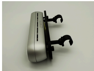
(b) Part 3 screwed to D455 camera.
